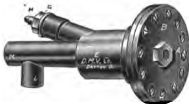
FIG. 209.—The "Dayton" Fuel Feed Regulator. This device differs from the others shown in that it has not two chambers necessitating that the valve rod pass through a packing gland. The cover, B, is attached to the end of the diaphragm chamber by small screws, but both may be detached, by threaded connection, from the spring and head chamber, thus avoiding removal of the diaphragm. The valve rod carries a needle valve controlling the gasoline inlet at M, and its outlet at L. The compression spring is adjusted by the stud, H, passing through the packing gland, G.
